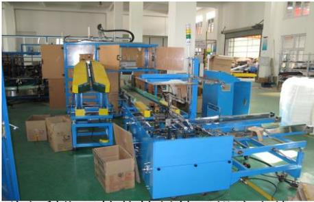
联合利华开箱装箱封箱码垛流水线
